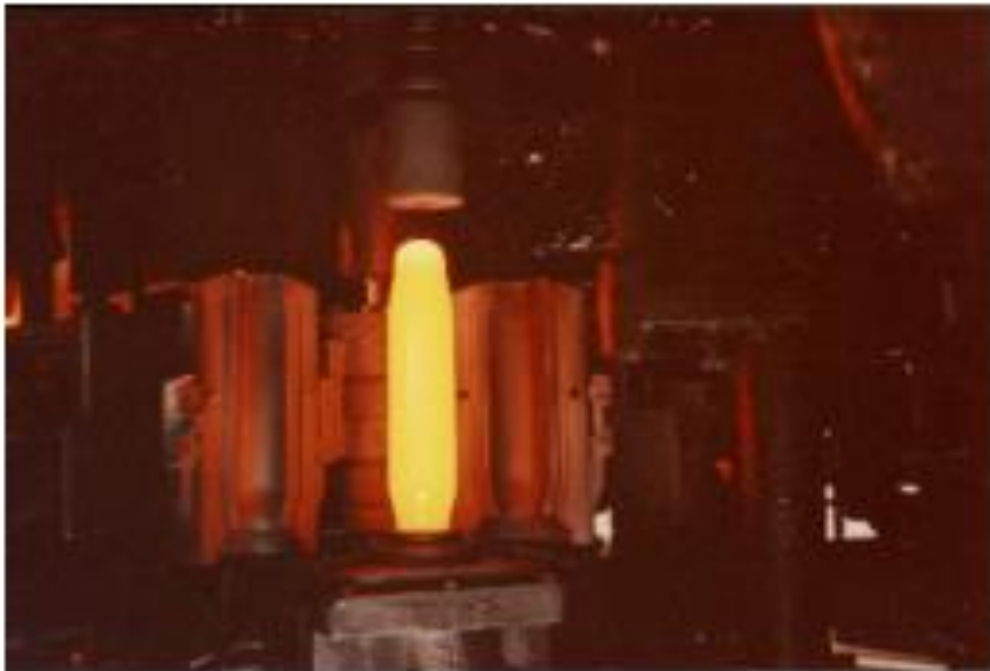
The parison machine at Lewis and Towers, Edenbridge, c1980. The mould is comprised of two halves.
