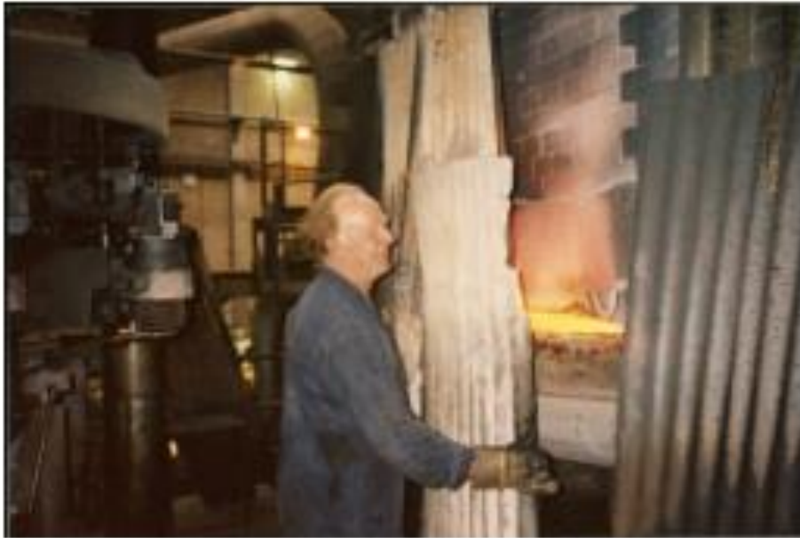
Arthur Brooks tending to the furnace at the Edenbridge plant, c1980. The required temperature for soda lime glass is 1000°C.
