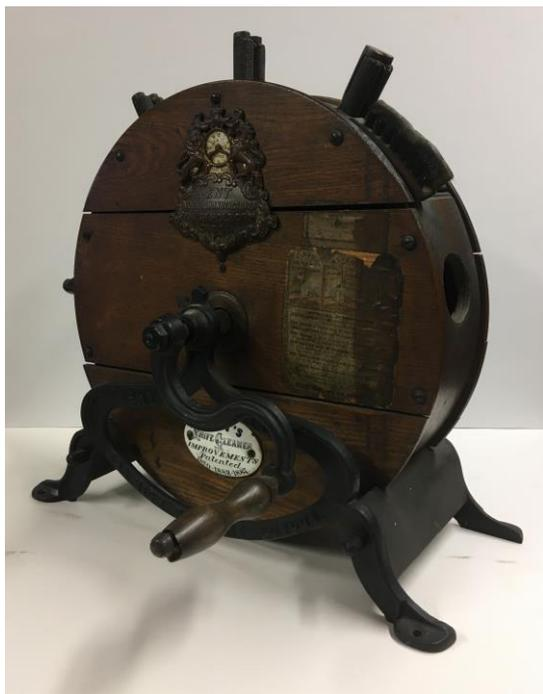
**Rotary knife cleaner made by George Kent Ltd. of High Holborn between 1887-1903.**
